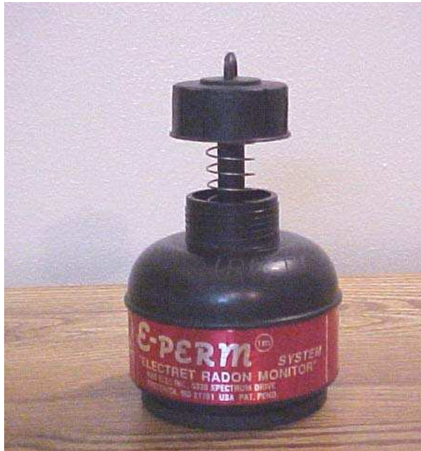
Short-term passive integrating device providing average radon concentration values
