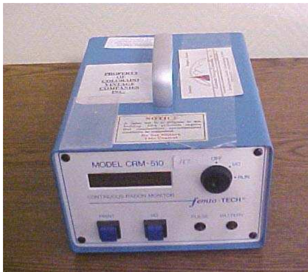
Continuous radon monitors providing average radon concentration values and hourly measurements
