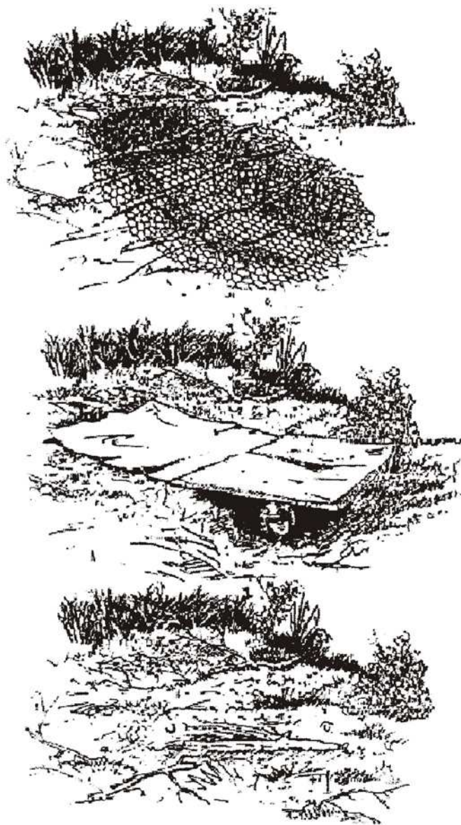
Figure 11-2: Construction of an OP—Option 1
